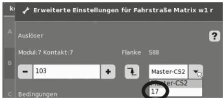
If everything has been entered correctly, confirm it with the green check mark. Store in memory along the way with the blue arrow on the display now appearing in the image. After that edit or process other routes or confirm with the green check mark and end the process.
